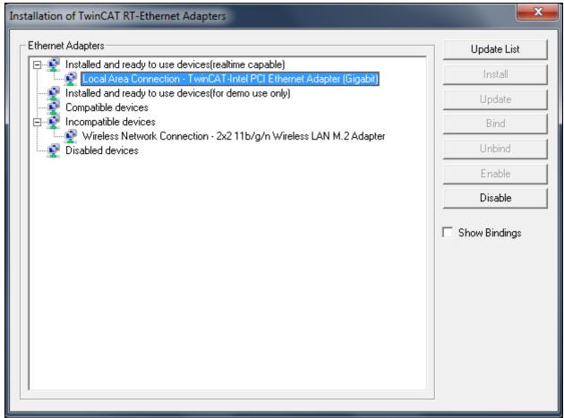
5. Go to the corresponding network adapter properties and then select TwinCAT drivers as displayed in Figure A-5 and Figure A-6. To access network adapter properties as seen in the figures below go to Control Panel\Network and Internet\Network Connections.
