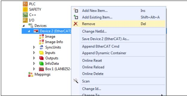
3. Scan for EtherCAT slave devices by right-clicking Devices under I/O and then selecting Scan, as displayed in Figure C-2.
