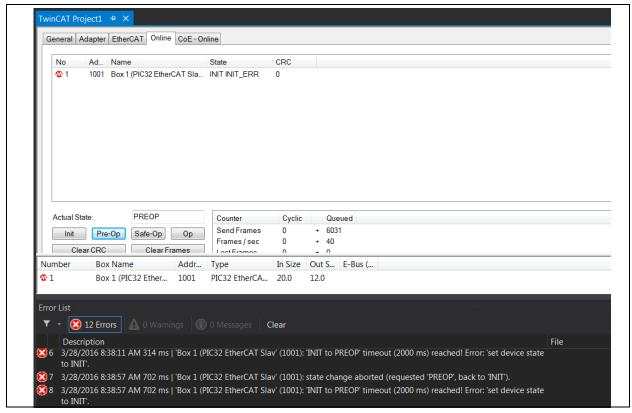
The board is not configured correctly to use the desired mode. Please refer back to Section 2.1.1 "EtherCAT Master and Slave Configuration" for information on the proper configuration of the board for HBI mode and Section 2.2.1 "EtherCAT Master and Slave Configuration" for information on the proper configuration of the board for SPI mode.
