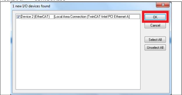
If the check box is not checked as displayed in Figure C-4, then either the device is not functional or the driver is not installed properly.
