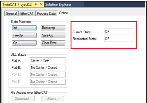
**Note:** If it changes to OP mode as highlighted above, then the device is in operational state. Otherwise there is an issue with the setup.
