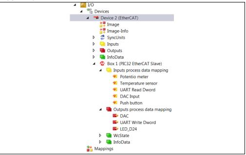
As part of this demo, eight object variables are mapped to PIC32 pins as detailed in Table 2-1.
